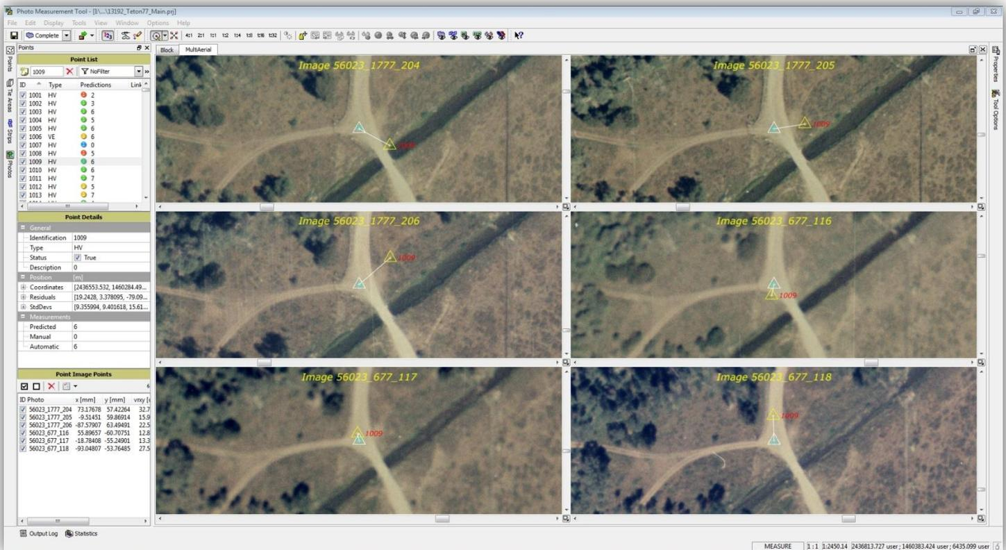
Trimble-Inpho's Match-AT software (Version 5.5) was utilized to perform fully analytical digital aero-triangulation. Manually measured tie points extended full control for each stereo model.
